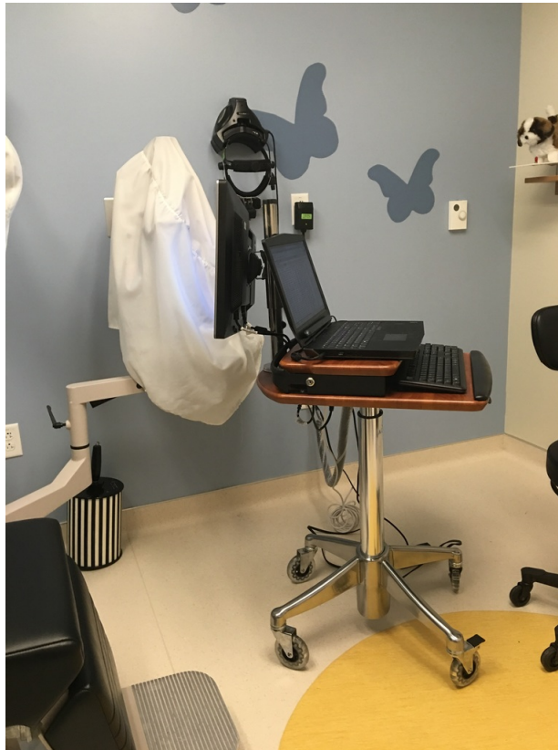
Figure 2: A photo of the Healthx mobile system. The table wheels can be locked down to prevent movement. The system has two screens: a laptop screen where the session operator can operate the playing session and the monitor where the player can interact with the game.
