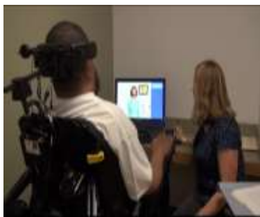
Figure 2. A user with Spinal Cord Injury interacting with the ECA on a 21" touchscreen. User input to the conversation is obtained via multiple choice selection of utterances. There is no speech input.
